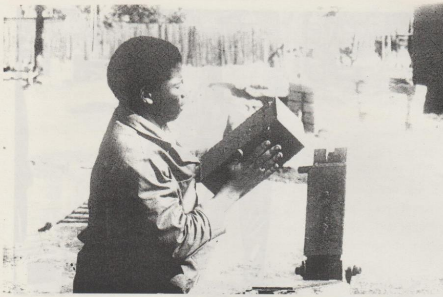
Figure 21 Removing the Block
